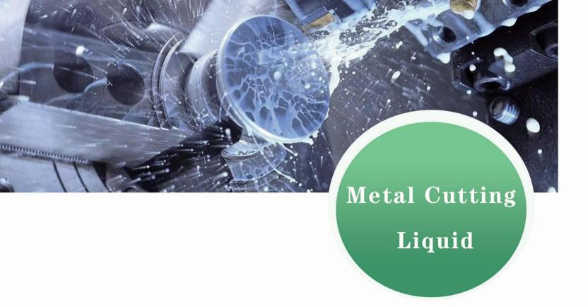
Metal cutting liquid contains fully-synthetic cutting fluid, semi-synthetic cutting fluid, emulsified cutting fluid, and oil cutting fluid. It's used to cool and lubricate the metal processing. Due to the high shear and functional additives, the foam is contributed. The unwanted foam can cause reservoir overflows, unplanned downtime and equipment damage.
